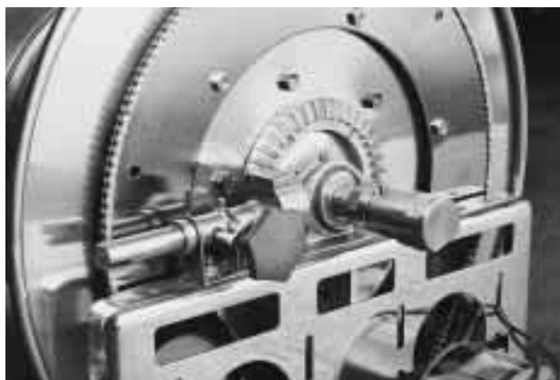
Ring and pinion shaft rewind unit with removable crank handle
